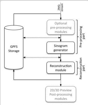
**Fig. 1** Diagram illustrating the main blocks and flow of the post-processing pipeline (*solid lines*). *Dash lines* indicate optional modules (e.g., phase retrieval) and actions (e.g., writing sinograms to file)
