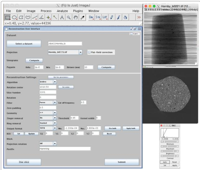
**Fig. 3** Graphical user interface (*large panel* on the *left*) enabling parameter optimization and job submission to a cluster facility for the reconstruction of full 3D volumes without the need for complex and error-prone command line activity. It is implemented as a Fiji plugin (Fiji main menu *top left*): all Fiji tools (e.g., contrast optimization tool *bottom right*) are available for projection (*top right*) and reconstruction (*middle right*) quality evaluation
