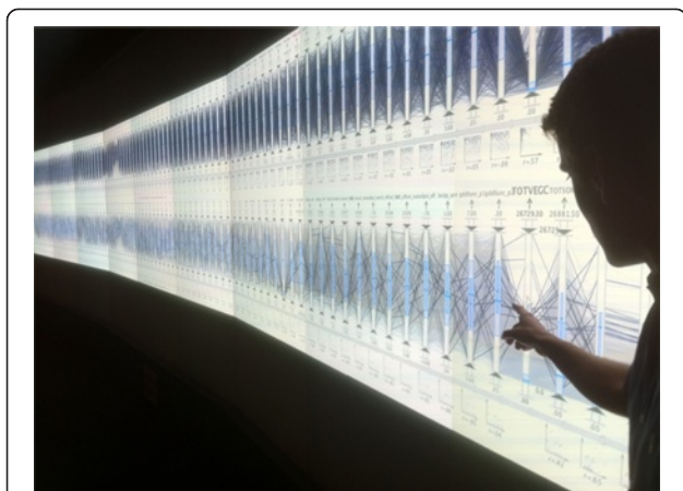
Figure 15 Lossless multidimensional visualization. EDEN is used to visually analyze a 1,000 simulation CLM4 point ensemble data set with 81 parameters and 7 output variables on ORNL's EVEREST power wall facility which offers 115,203,072 (35 million) pixels. EDEN is a promising technique for materials science data analysis especially when it is coupled with dimensionality reduction and statistical learning algorithms.
